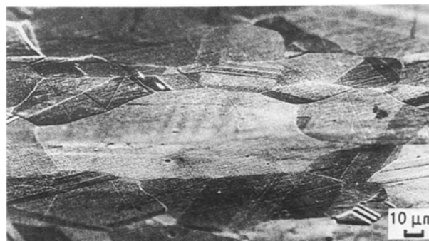
Figure 5 Scanning electron micrograph of a grain assembly (i.e. a large grain plus the surrounding small grains) of the 70/30 brass annealed at 600 °C. Of the 21 small/small grain boundaries 10 were found to be CSL boundaries while no CSL boundaries could be found between the large and the small grains.
